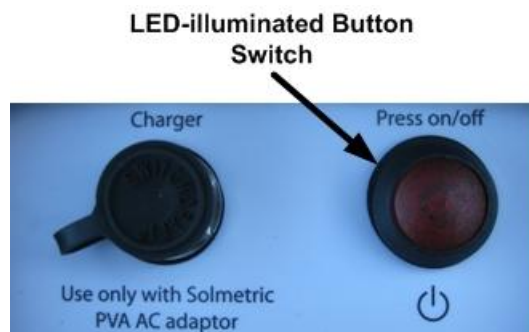
Figure 9. Powering-up the I-V Measurement Unit
