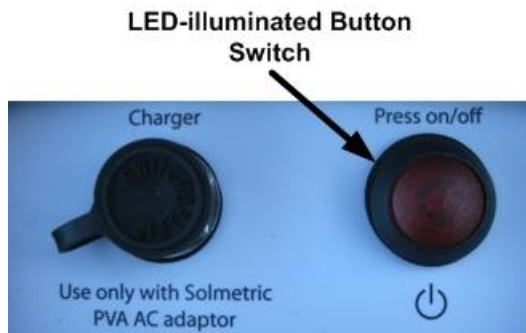
Figure 33. Turn on the I-V Measurement Unit
