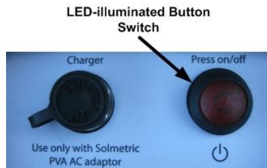
Figure 6. LED-illuminated button switch
