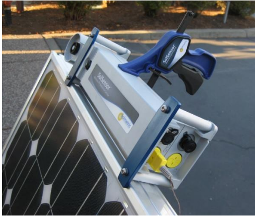
Figure 12. SolSensor mounted on the frame of a PV module
