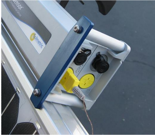
Figure 16. Thermocouple plugged into the TC1 connector.
